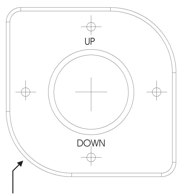
Wires exit here for proper orientation.
